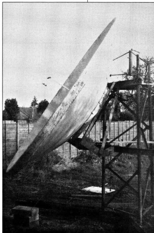
Fig. 2: The simple solid dish, mounted on a small tower for the G3WDG/G4KGC e.m.e. experiments.
